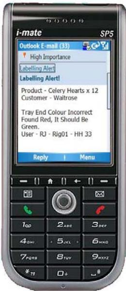
Fig 1. SMS Failure Alert TXT Message, showing; product, customer, reason for failure, user, location where test was completed and which handheld was used.
